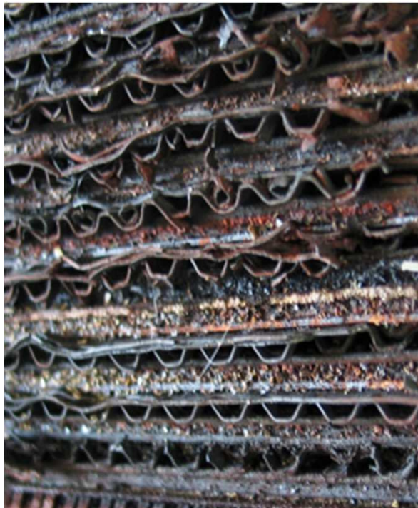
MCFC stack corrosion by halogenated HCs
