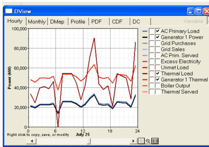
Figure 12: Operation of the biomass CHP plant in a summer day (output of Homer software)
