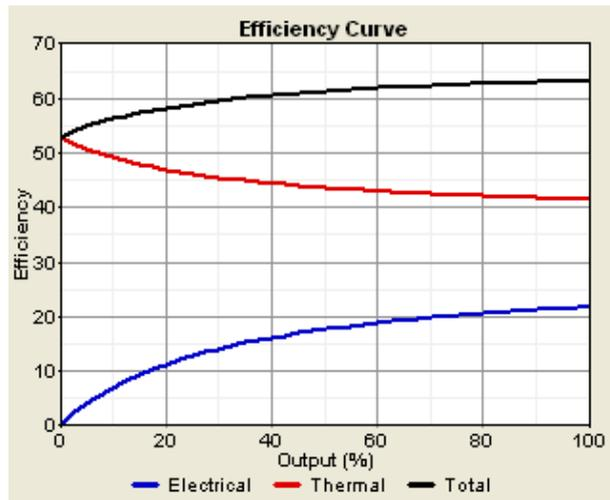
Figure 10: Electric and thermal performances assumed for the biomass CHP plant
