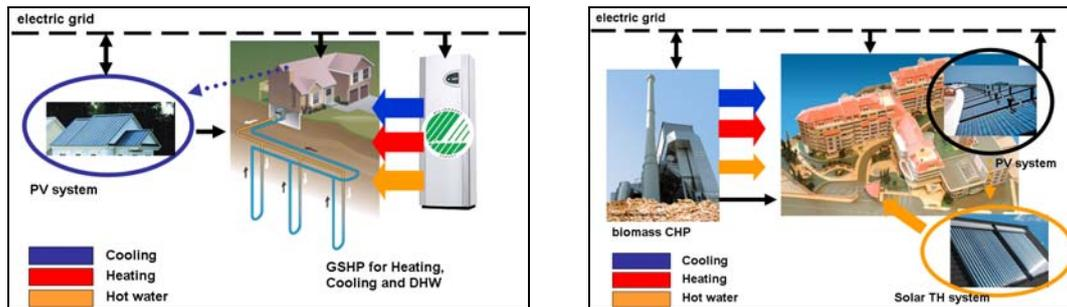
Figure 6: Energy supply for villas (left) and other residential buildings (right)
