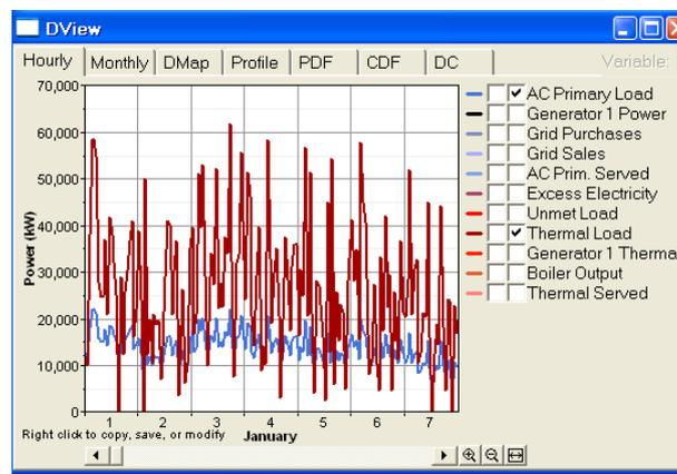
Figure 9: View of the hourly calculations by Homer (thermal and electricity demand in January); <http://www.nrel.gov/homer/>
