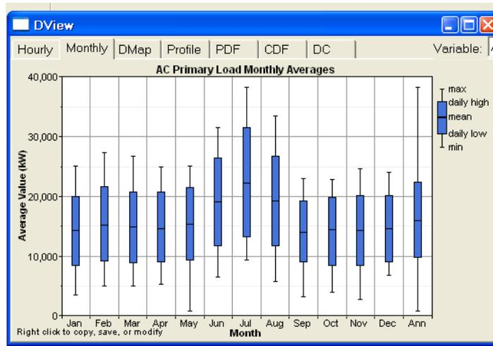
Figure 11: Electricity demand met by the biomass CHP plant (summer peak due to compression chillers for cooling)
