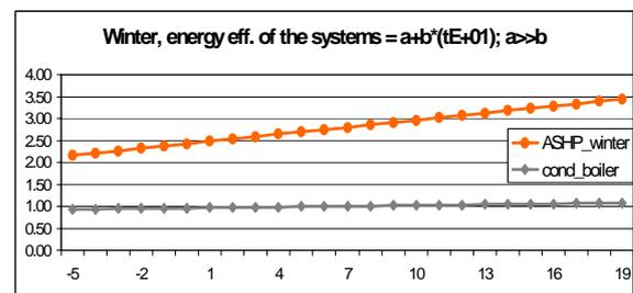
Figure 1. Curves of the energy efficiencies, heating systems
