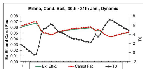
Fig. 5. Example of hourly trend of exergy efficiency (as absolute values) vs.  $T_0$  and Carnot factor (Milano, heating by condensing boiler)
