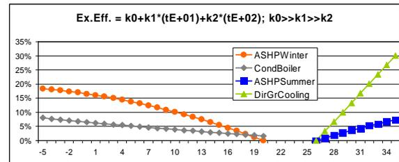
Figure 3. Curves of the exergy efficiencies; dependence on  $T_0$  could be approximated as a second order relation (with system depended coefficients)
