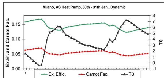
Fig. 4. Example of hourly trend of exergy efficiency (as absolute values) vs.  $T_0$  and Carnot factor (Milano, heating by ASHP)
