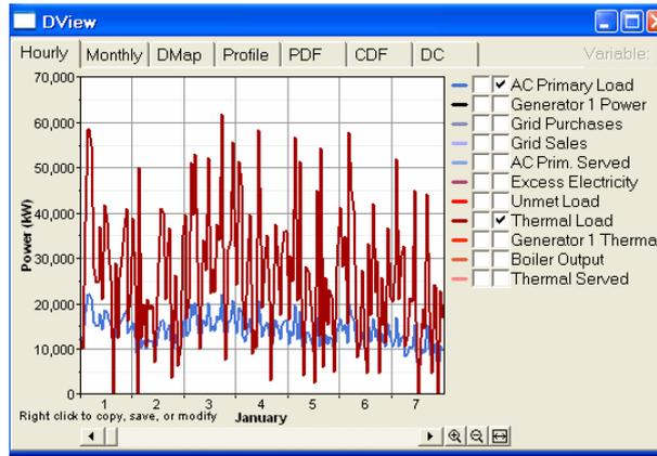
**Figure 9: View of the hourly calculations by Homer (thermal and electricity demand in January);**
