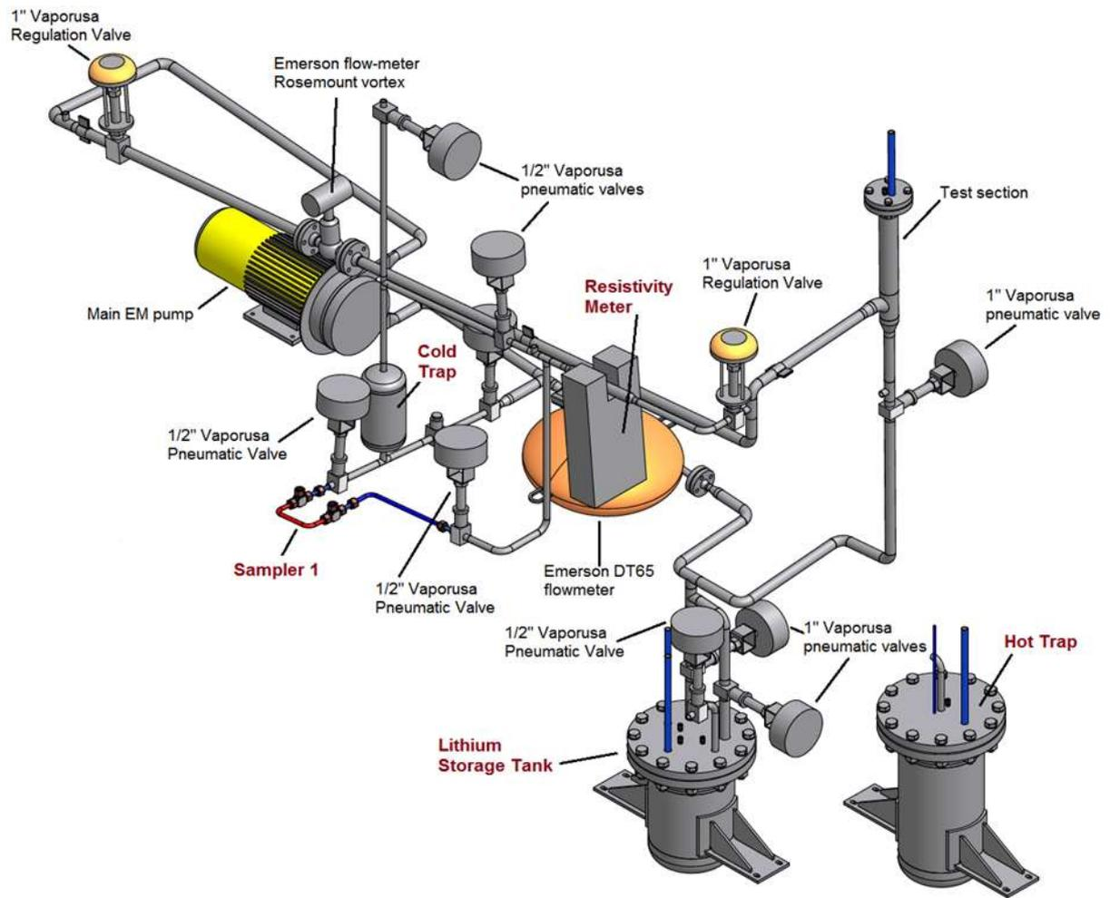
Figure 1 - Lifus 6 main loop 3D configuration
