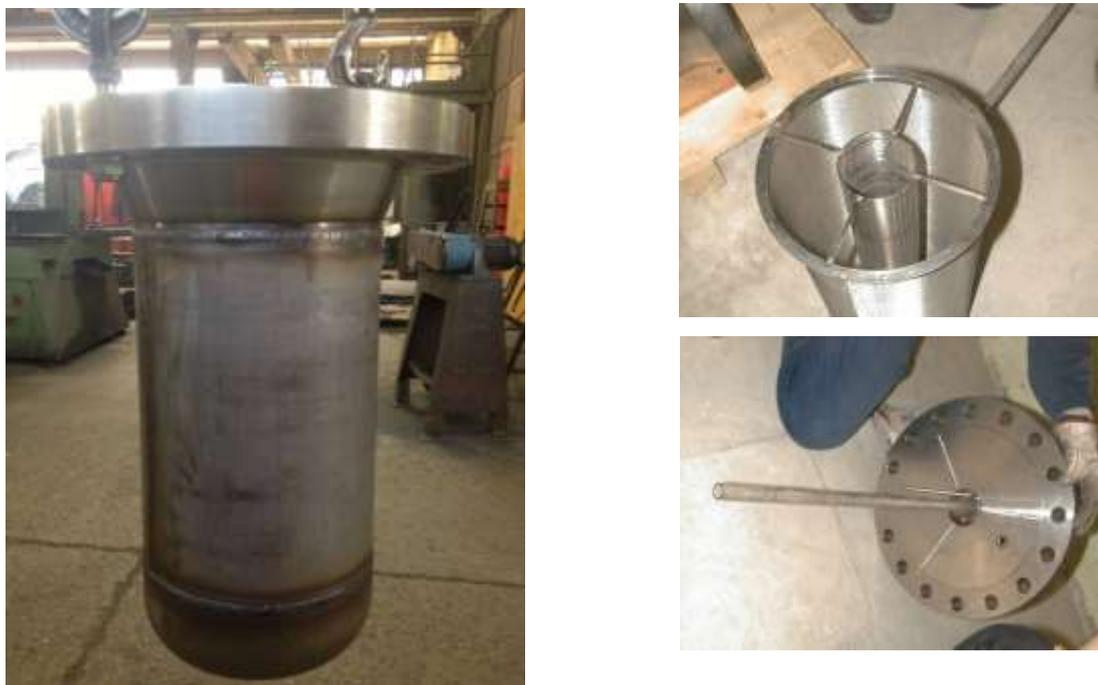
Figure 9 - hot trap assembly
