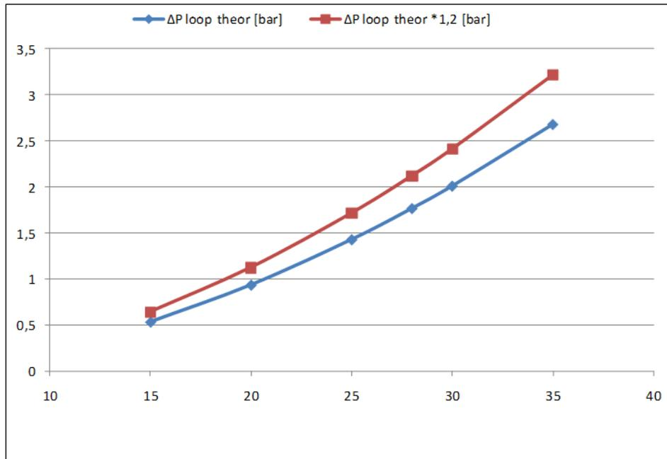
Figure 3 - Theoretical hydraulic characteristic of the selected pump
