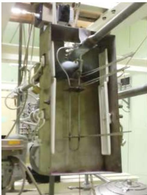
Figure 8 - R-meter installation on the purification branch
