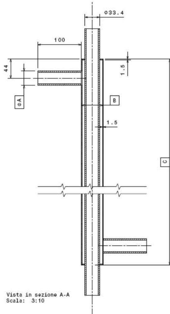
Figure 5 - design of the lithium/air heat exchanger
