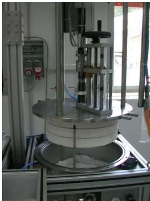
Fig. 5-3 – Experimental chamber: detail of the flange with the sliding and rotating system.
