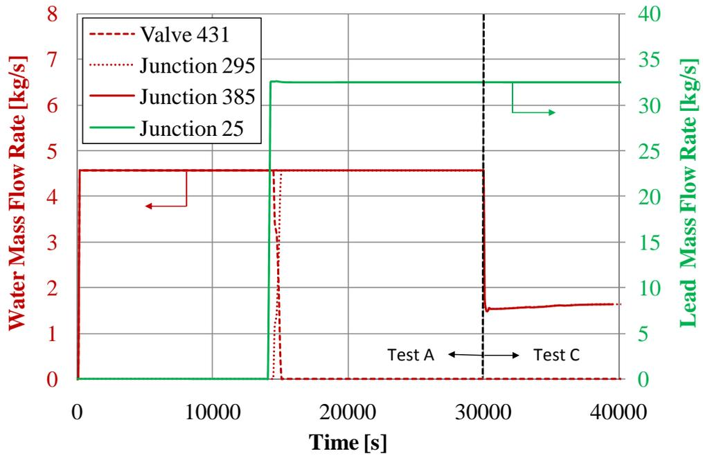
Figure 10. Mass flow rate in the primary and secondary side of HELENA facility (Test A + Test C)
