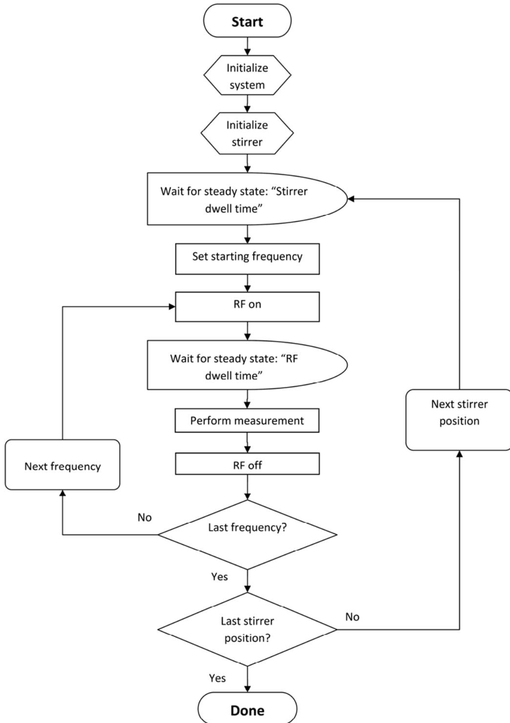
**Fig 7:** Measurement flow diagram.
