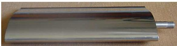
In fact corrosion and wear resistant composite coatings have been realized by electrochemical co-deposition of ENEA SiC NPs with different matrix materials (nickel or bronze) on steel
