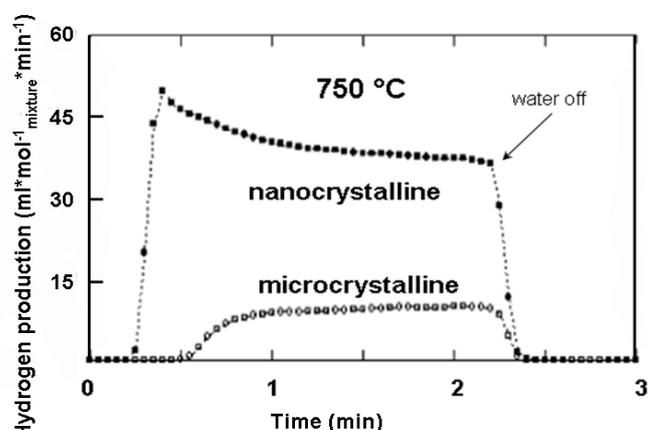
Figure 1. Hydrogen generation rate from water utilizing microcrystalline and nanocrystalline  $\text{MnFe}_2\text{O}_4$  blended with  $\text{Na}_2\text{CO}_3$ .
