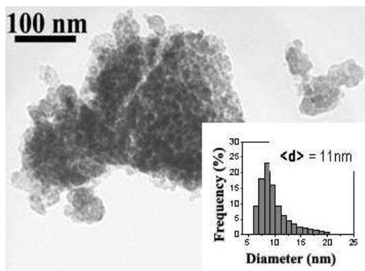
Figure 2. TEM micrograph of MnFe<sub>2</sub>O<sub>4</sub> nanoparticles synthesized in a water-in-oil micellar systems.
