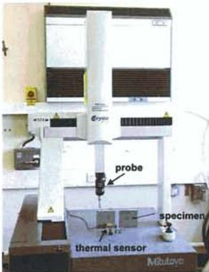
Coordinate measuring machine used for the contour method
