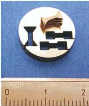
Micro-tensile weld specimens
