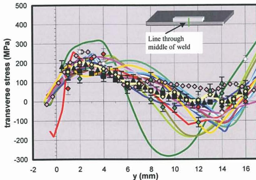
The figures show 18 FE predictions (solid lines) from 6 partners and 8 sets of measurements (symbols) including 6 neutron diffraction, deep hole drilling and contour method results; the upper graph gives transverse residual stress along a line 2mm below the plate surface and the lower shows the variation through the thickness at mid-length of the weld bead.
