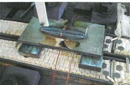
A more manageable 'auxiliary specimen' was manufactured with just three beads deposited in a slot within a 2.25CrMo ferritic steel plate ( $400 \times 200 \times 20$ ) mm<sup>3</sup>. Residual stress measurements have been obtained for this specimen using neutron diffraction and the contour method. Preliminary FE results have been obtained, and further work is being undertaken to incorporate phase transformation behaviour in the calculations.
