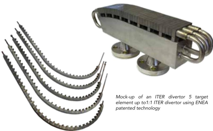
Mock-up of an ITER divertor 5 target element up to 1:1 ITER divertor using ENEA patented technology
