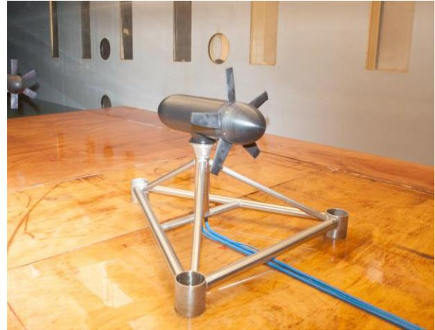
Fig. 2 Left: 1.5 m diameter model turbine during wave/current interaction tests in the wave tank (Courtesy Schottel Hydro GmbH); Right: Two 0.4 m model turbines during simulated turbine operation in array in the Circulating Water Channel (Courtesy SABELLA SAS)
