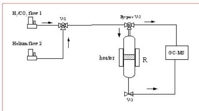
**FIGURE 1** Schematic of the measurement apparatus
